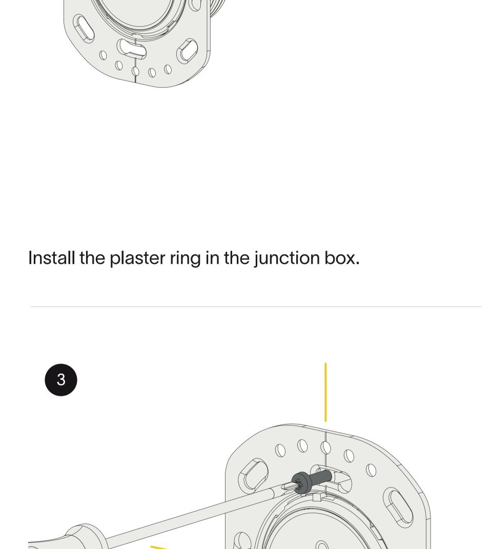
Level the plaster ring and fasten the screws.
